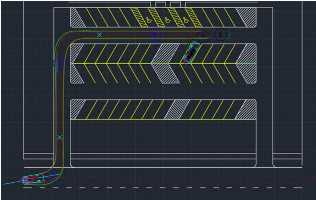
Typical passenger vehicle backing out of a parking stall and exiting the parking lot through the access road exit.
