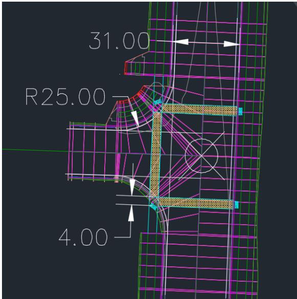
FIGURE 1A: INTERSECTION DETAIL WITH BRICK CROSSWALK
