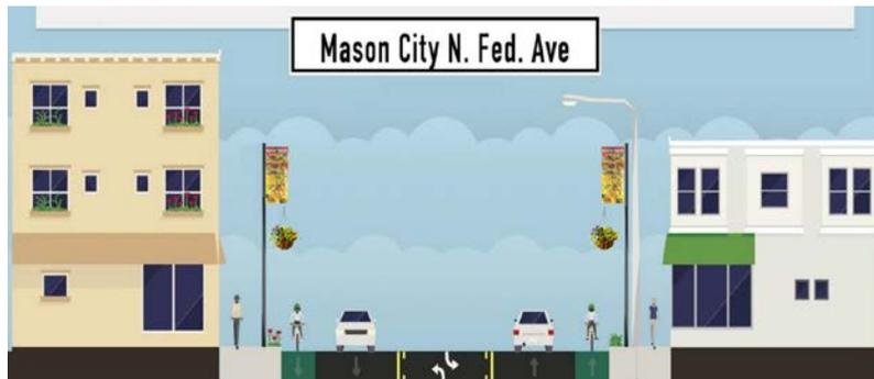
Figure 5.13. N. Fed. Ave. after resurfacing. This image shows those 5 feet wide clear zones transformed into bike lanes.
