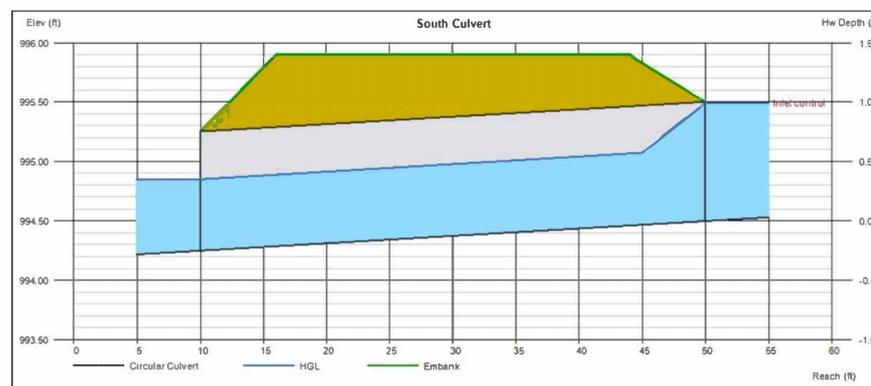
Figure 7: Culvert on south side of Road A
