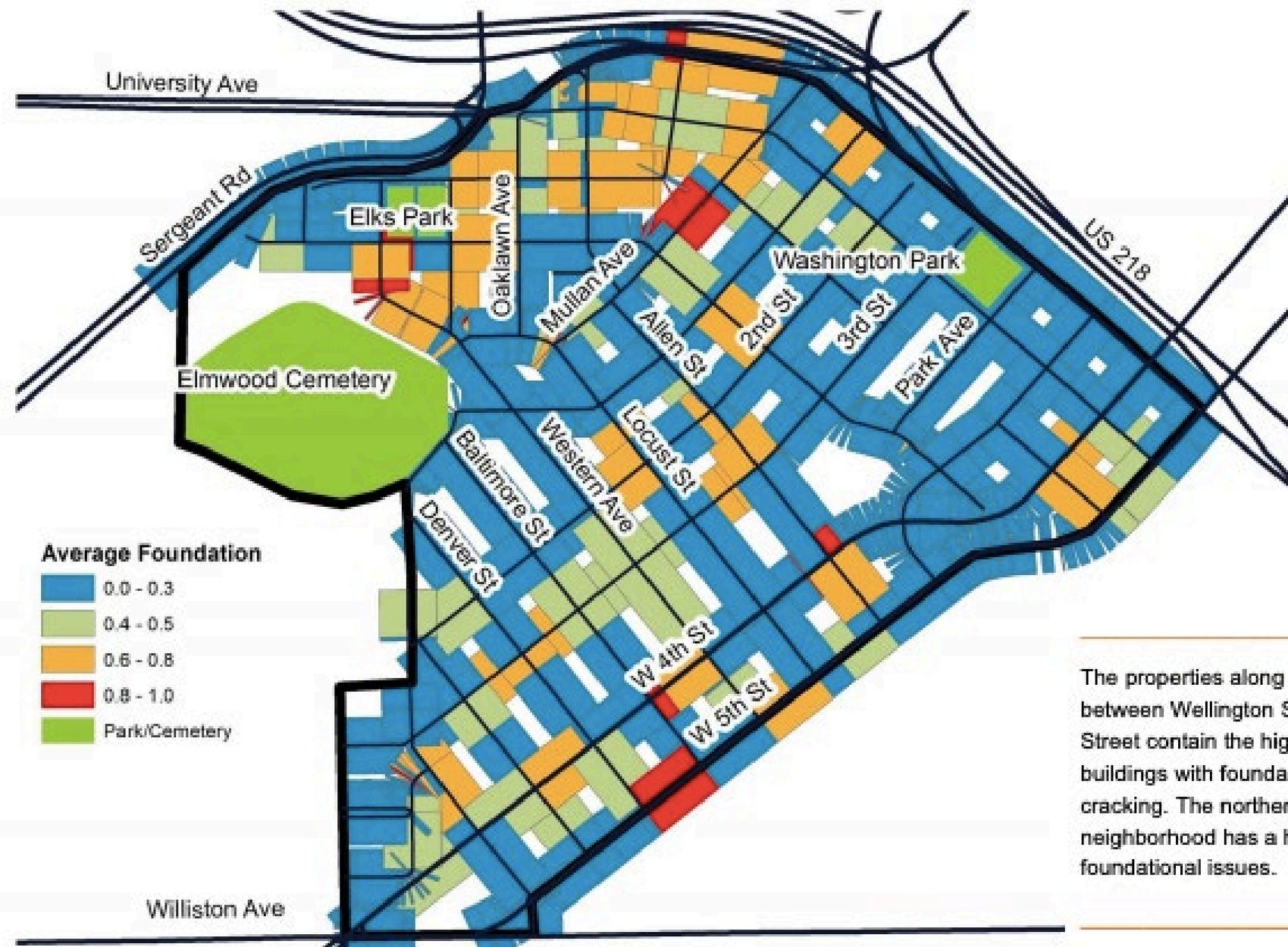
The properties along Mullan Avenue between Wellington Street and South Street contain the highest concentration of buildings with foundational slumping or cracking. The northern section of the neighborhood has a high concentration of foundational issues.
