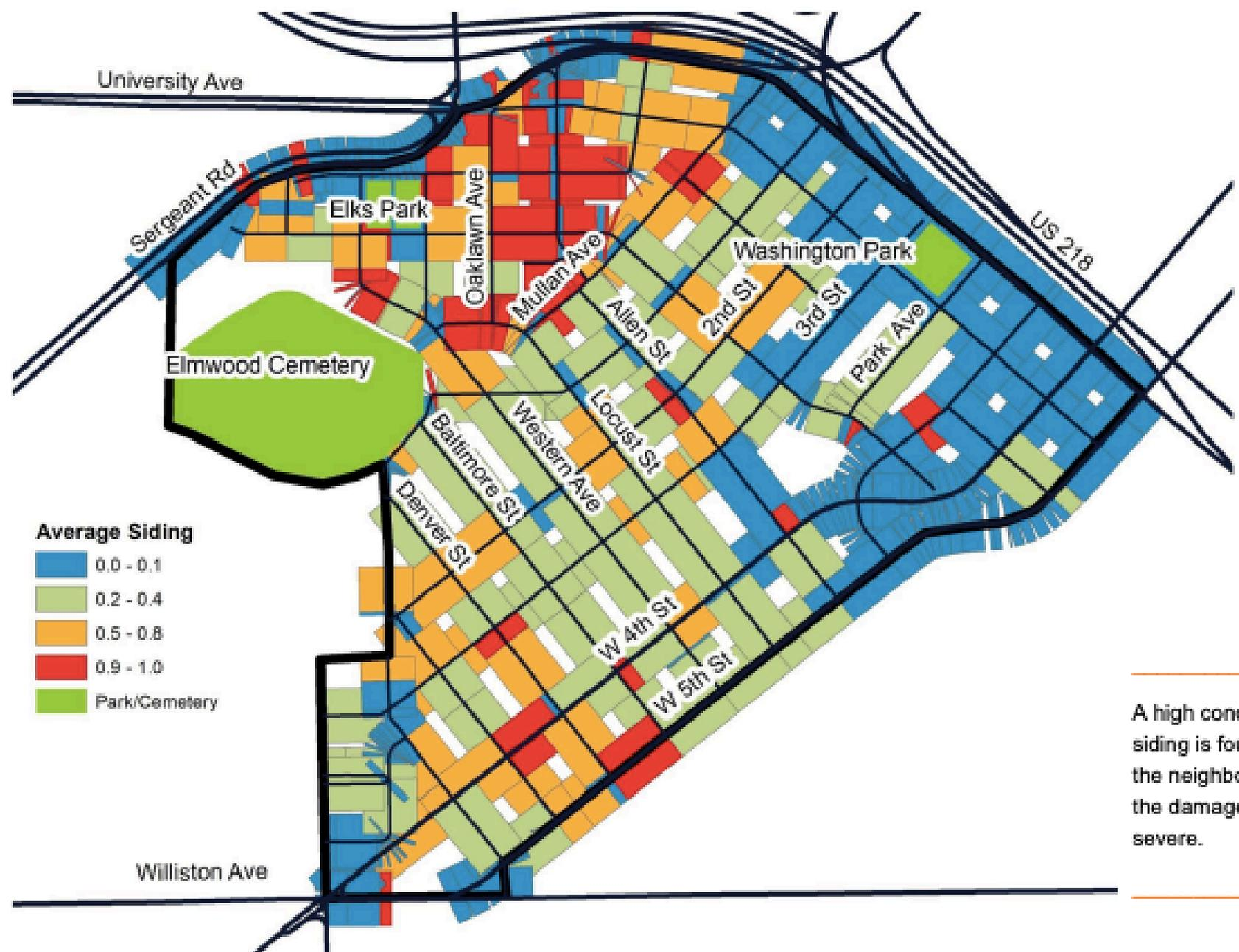
A high concentration of broken or molding siding is found in the northeast corner of the neighborhood. It should be noted that the damage seen on most homes was not severe.
