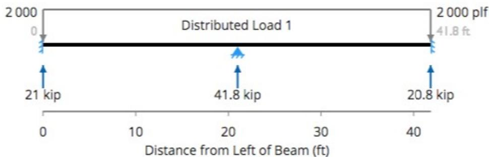
$$R_{left} := 21 \text{ kip} \quad R_{mid} := 41.8 \text{ kip} \quad R_{right} := 20.8 \text{ kip}$$
