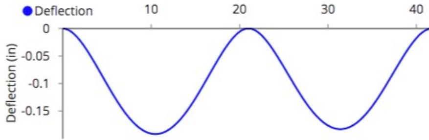
$\delta_{max} := -0.192 \text{ in}$   $\leq$   $0.25 \text{ in}$  Design is adequate.
