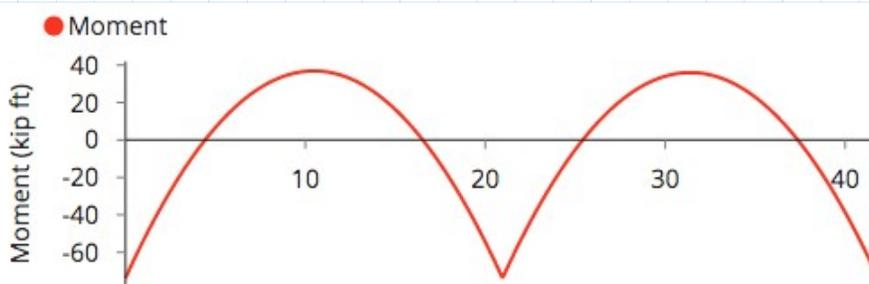
$$x := 0 \text{ ft} \quad M_u := M_{left} + R_{left} \cdot x - w_{self} \cdot \frac{x^2}{2} = -73.8 \text{ kip} \cdot \text{ft}$$
