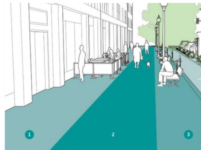
include things like lighting, kiosks, trees, and bicycle parking. This section acts as a protective buffer between sidewalk and street uses.
