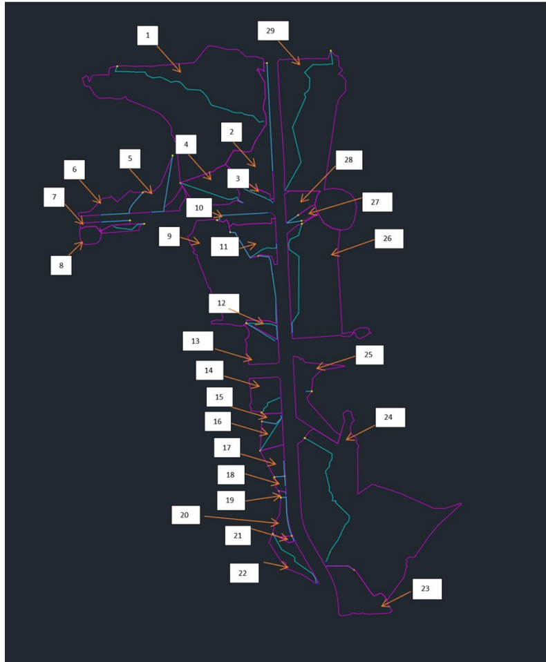
Figure 8: Screenshot of Civil 3D generated Catchments along the new roadway extensions, including flow paths from which time of concentration was determined.
