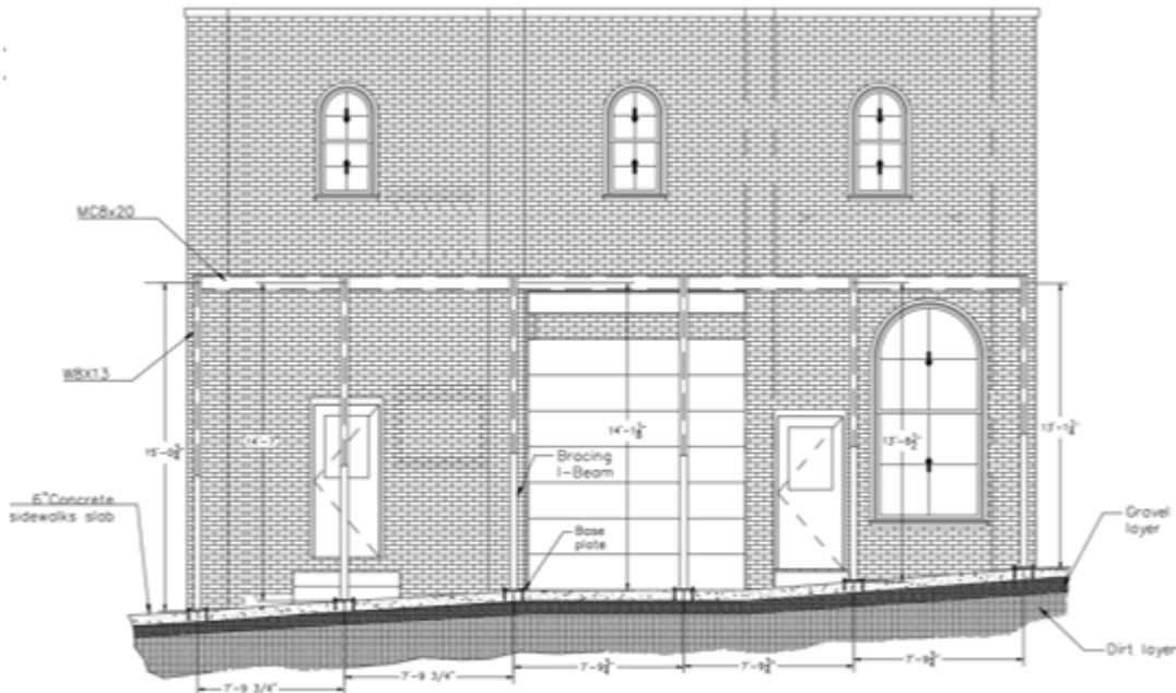
Figure 10: Elevation View of Bracing
