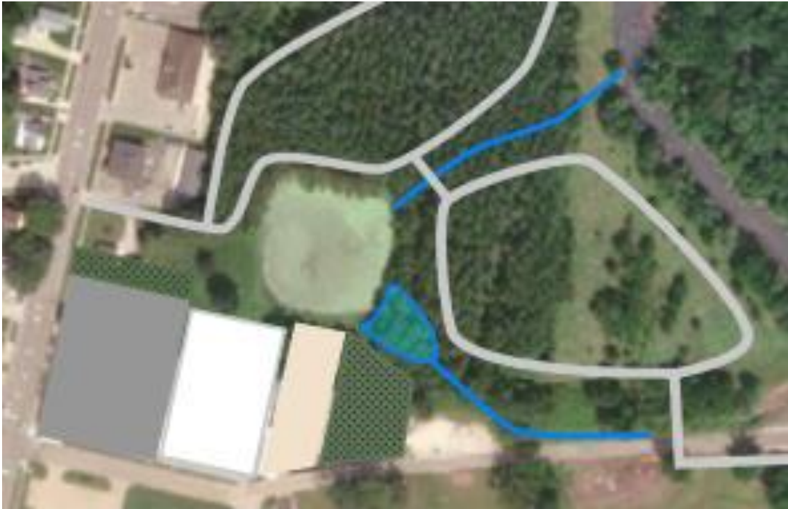
Figure 3 – Alternative stormwater design considered for 12-acre site.
