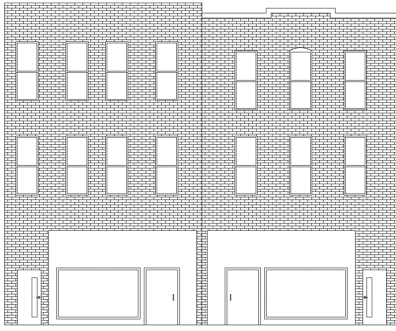
Figure 14: The front of the building after the facade is removed and the brick is restored to its original condition.
