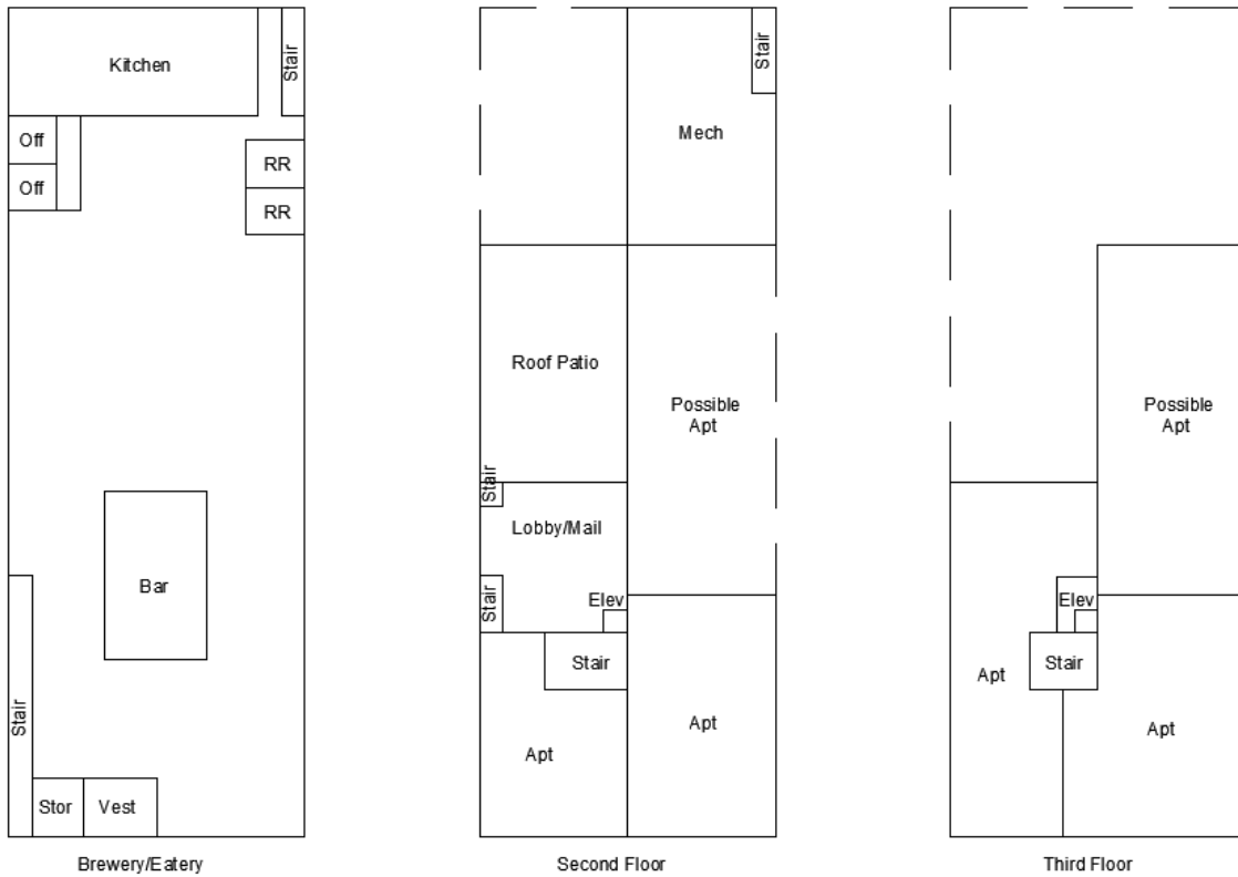
Figure 7: Alternative solution for the first floor being a brewery/eatery. The second floor being apartments with a lobby, elevator, roof patio, and mechanical room. And the third floor being apartments with an elevator.
