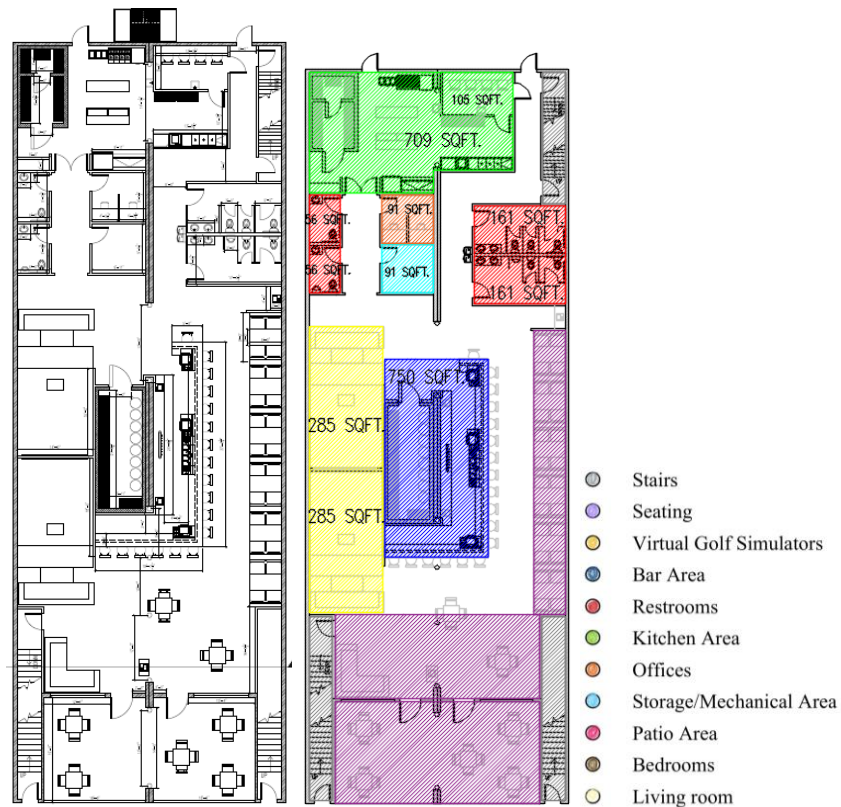
Figure 15: Final First Floor Architectural Layout
