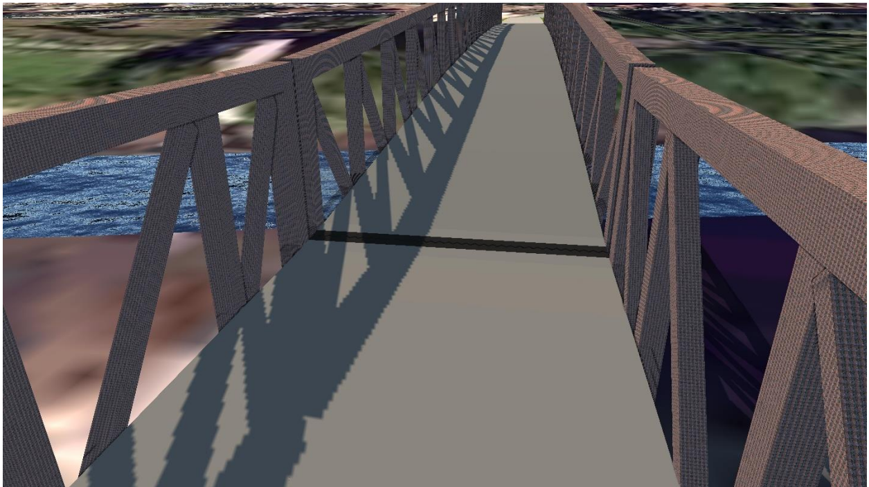
Figure G.6. 3D rendering pedestrian view looking west, showing the expansion joint.
