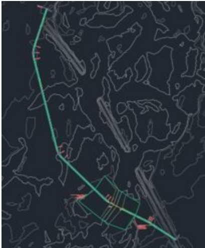
Figure 13: Alignment for the Western Trail Alignment in Civil 3D
