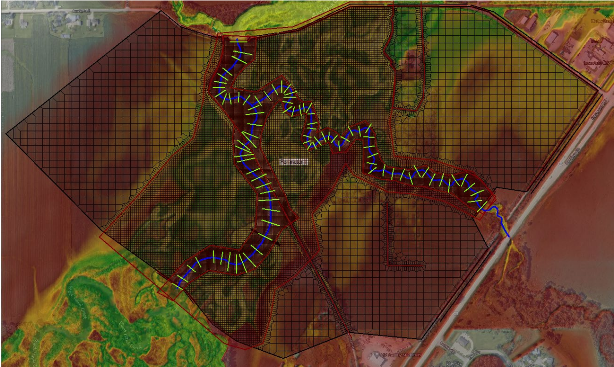
Figure 29: Model showing computational mesh with breaklines, refinement regions and boundary condition lines, as well as cross-sections used to create channel modifications
