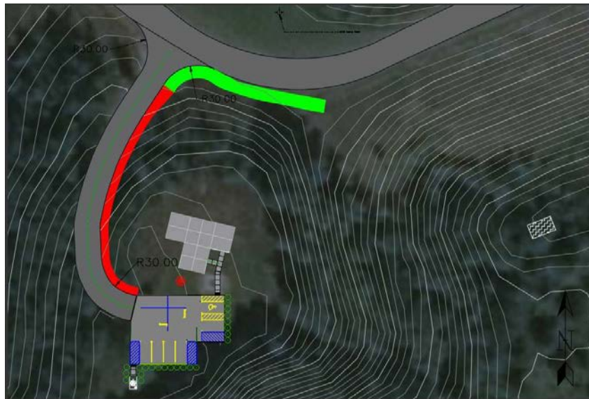
Figure 5: Two sod lined open channels
