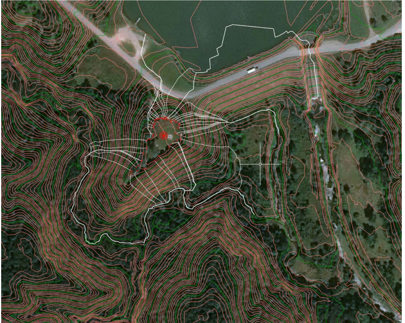
Figure 9: Drainage pre development
