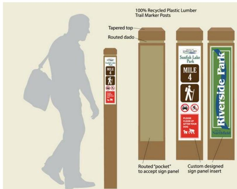
**Figure 10:** Recycled plastic lumber mile marker posts, courtesy of Vacker Signs Inc.
