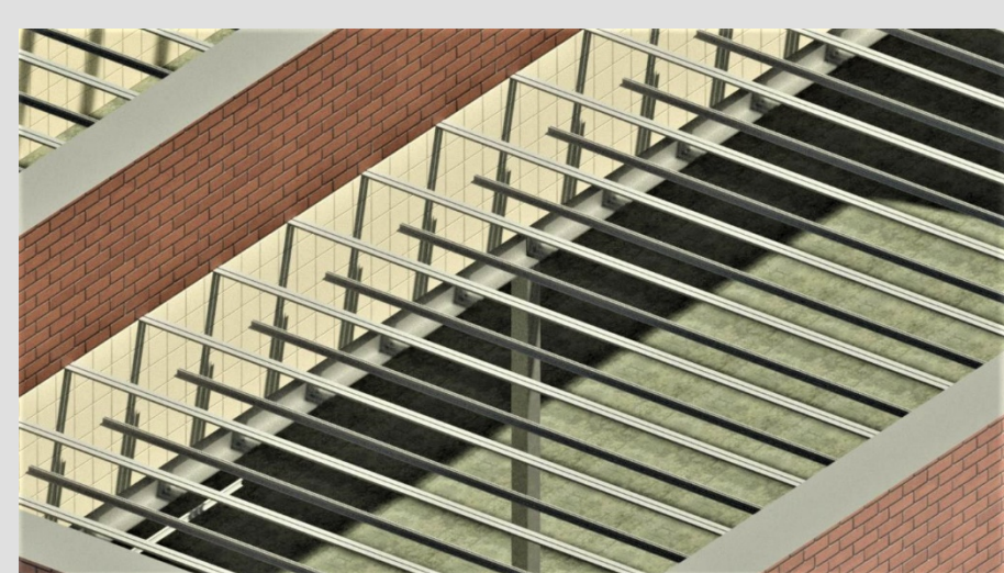
Figure 17: Structural cross-section of new roof
