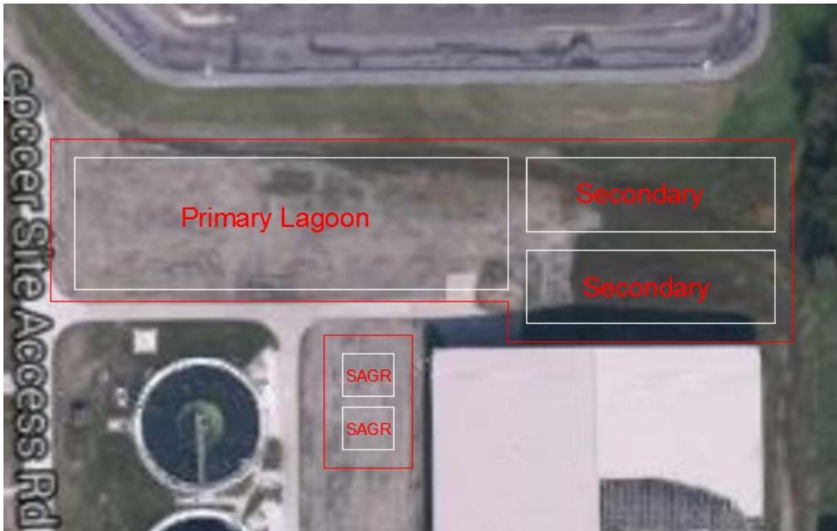
Figure 5: Final Design Layout of Lagoon and SAGR System
