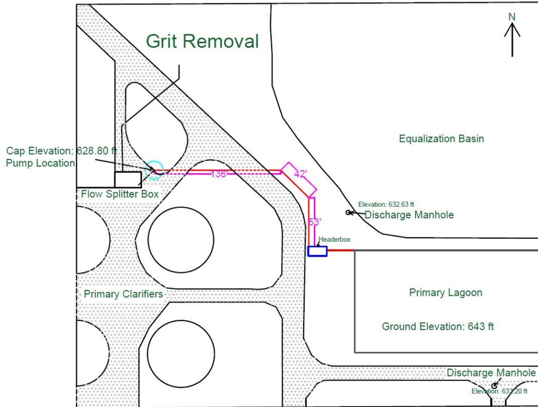
Figure 6: The piping network design option 1 layout. The pipes are shown in red, the light blue circle indicate the starting point and pump location, and the magenta lines are length measurements. The headerbox is the royal blue rectangle.
