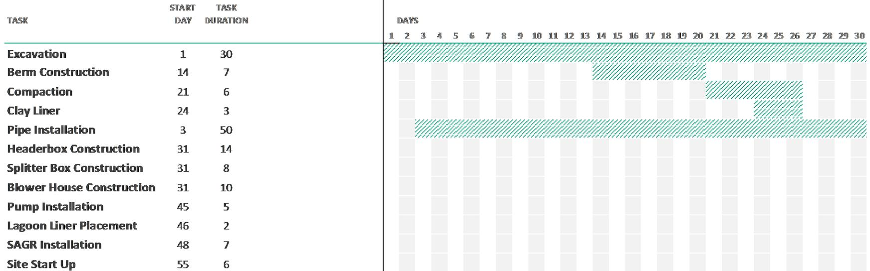
Figure 16: Gantt chart of the first 30 days of estimated time of construction for the SAGR System
