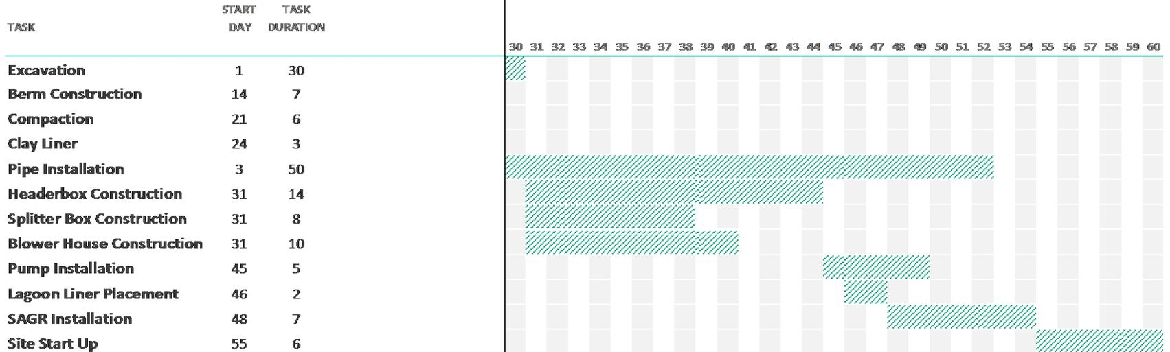
Figure 17: Gantt chart of the last 30 days of estimated time of construction for the SAGR System
