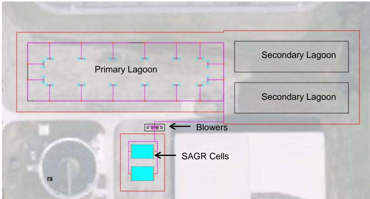
Figure 11: Overall Blower System Layout
