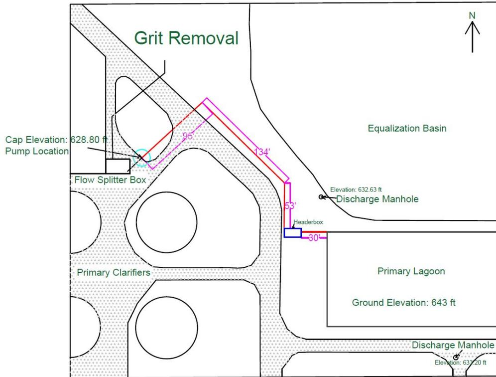
Figure 7: The piping network design option 2 layout. The pipes are shown in red, the blue circles indicate the starting point and pump location, and the magenta lines are length measurements. The headerbox is the royal blue rectangle.
