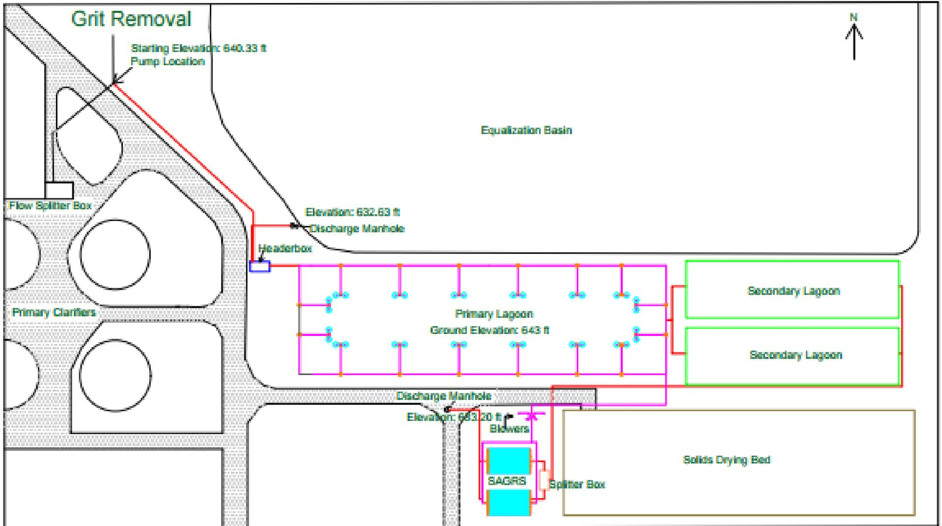
Figure 14: Final Pipe and Lagoon Design
