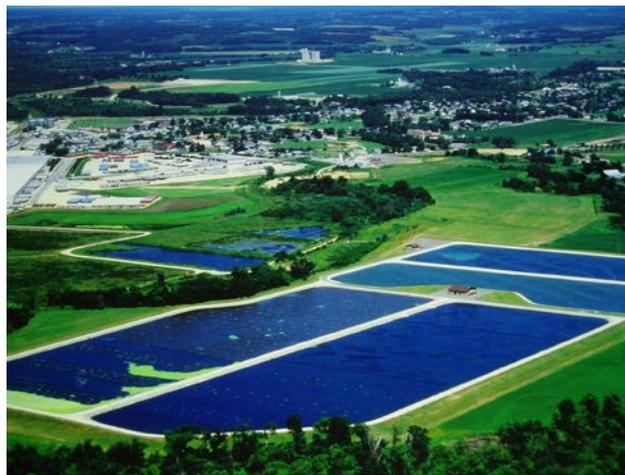
Figure 4: A wastewater treatment lagoon with submerged aerators
