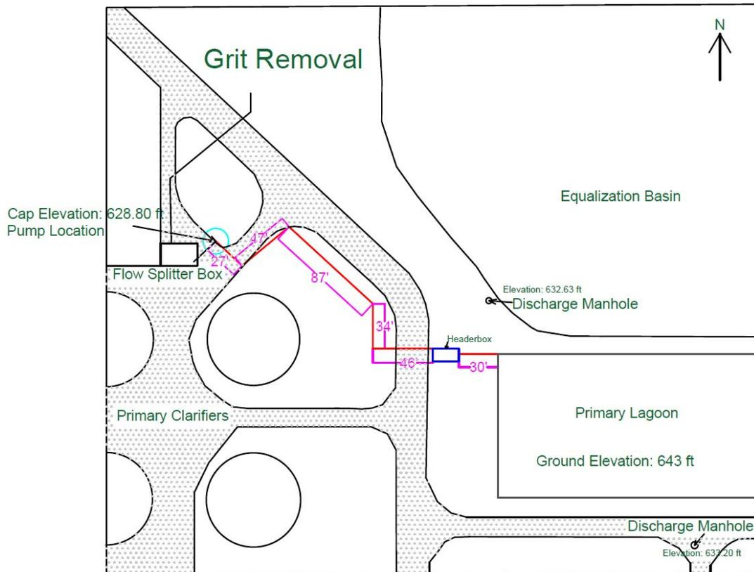
Figure 8: The piping network design option 3 layout. The pipes are shown in red, the blue circles indicate the starting point and pump location, and the magenta lines are length measurements. The headerbox is the royal blue rectangle.
