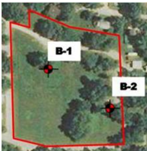
Figure 7. Image showing the location of borings where Terracon took samples during the Limited Site Investigation.
