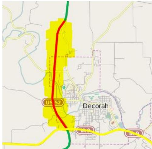
Figure 1: Pavement Condition (based on IRI) for U.S Highway 52 (highlighted in yellow) from Iowa DOT. (Good = green, Fair = yellow, and Poor = red)
