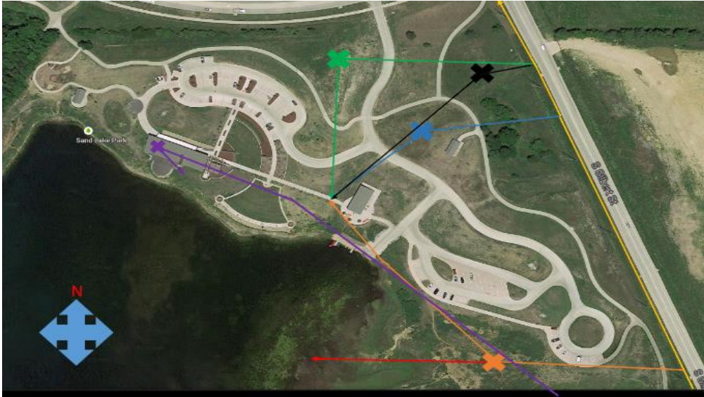
Figure 5: Terry Trueblood Recreation Area alternative 2. Each colored 'X' depicts a possible reservoir location and its associated pipelines to be constructed. The red line marks another potential pipeline which would deliver water to Sand Lake.
