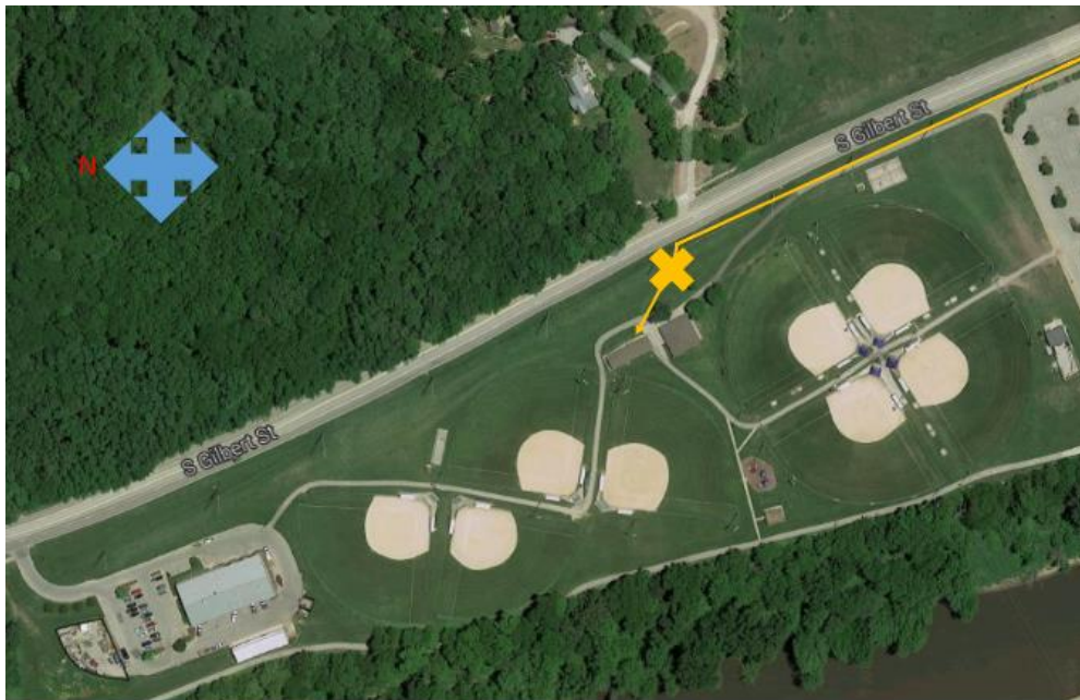
Figure 6: Napoleon Park alternative 2. Water is directed from the force main to the reservoir to the main irrigation building by a new pipeline, where it will be distributed to the softball fields.
