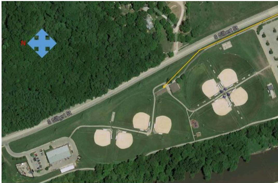
Figure 4: Napoleon Park alternative 1b. Water is directed from the force main to the main irrigation building by a new pipeline, where it will be distributed to the softball fields.
