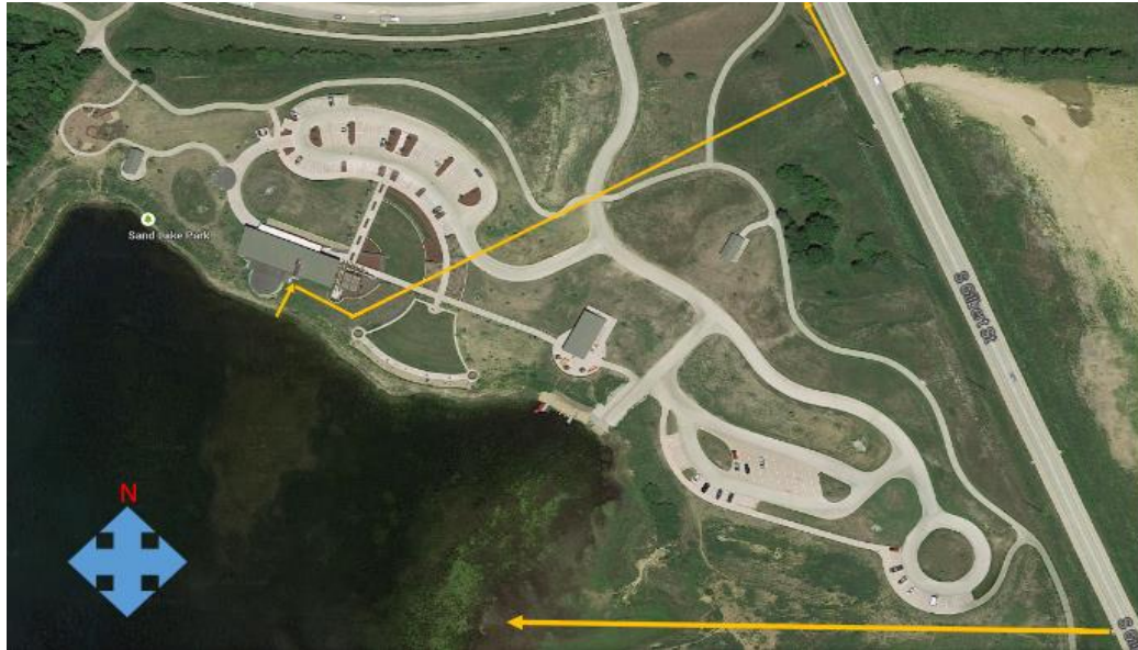
Figure 1: Terry Trueblood Recreation Area alternative 1a. Effluent from the ICWWTPS will enter Sand Lake at the South end. Water will be withdrawn from the lake south of the lodge, at the north end of the lake. A pipeline will be installed from the lodge back to the force main, where it will be carried to Napoleon Park.
