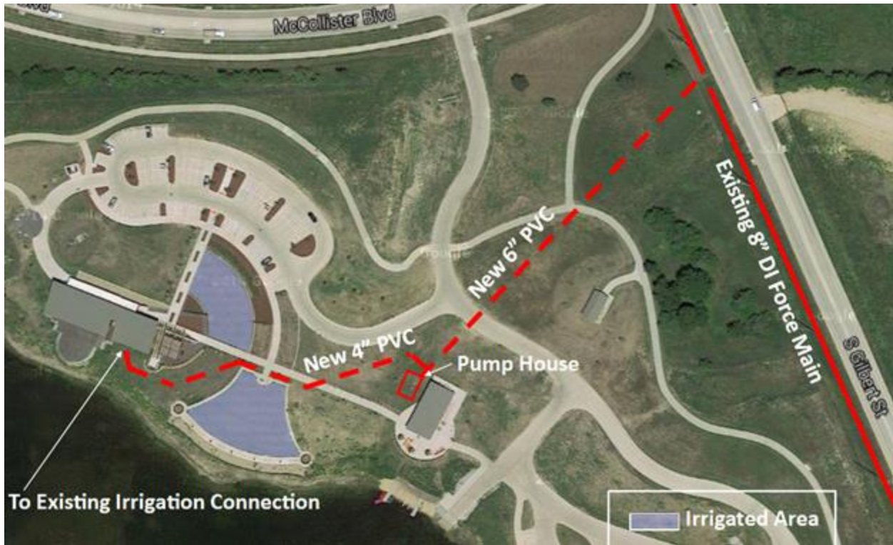
Figure 19: Pipe layout of the piping system at the Terry Trueblood Recreation Area
