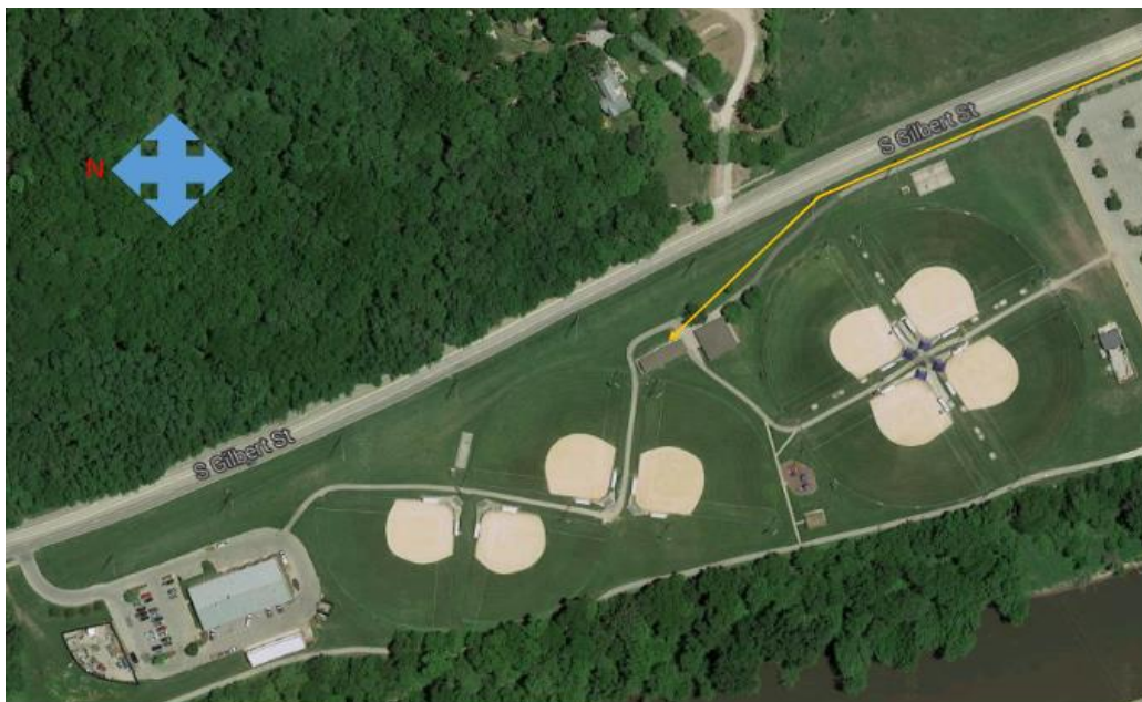
Figure 8: Napoleon Park alternative 3. Water is directed from the force main to the main irrigation building by a new pipeline, where it will be distributed to the softball fields.
