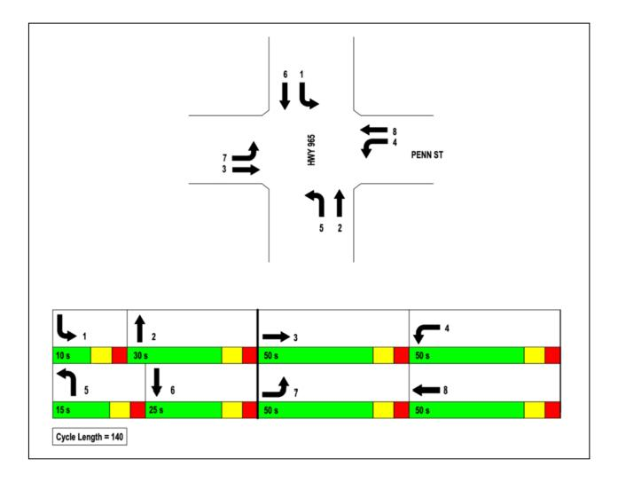
Figure 11: Phasing and Timing Plan.
