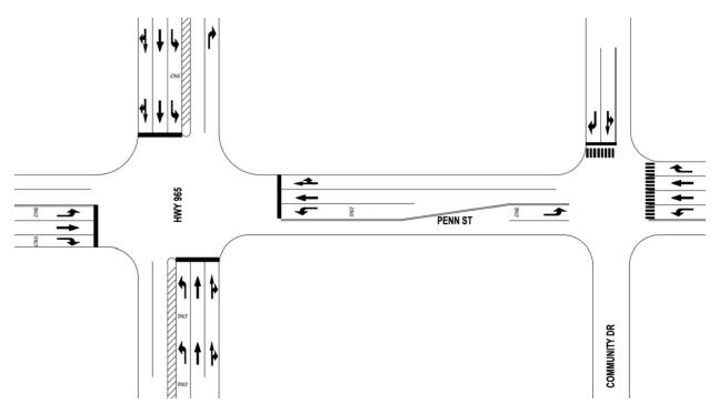
Figure 13: Widening the right of way alternative illustration.
