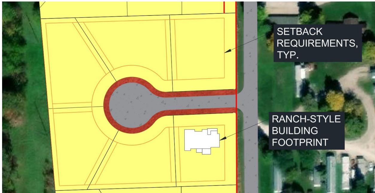
Figure 6.5. Civil3D lot layout with setback offsets and representative building footprint
