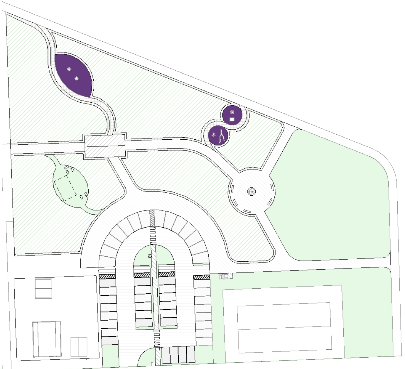
Figure 7: N River St. Site phase 6 site plan including all construction from previous phases. Major features include Farmer's Market parking lot structure, trail network through the prairie, pavilion, and three recreation spaces for families.
