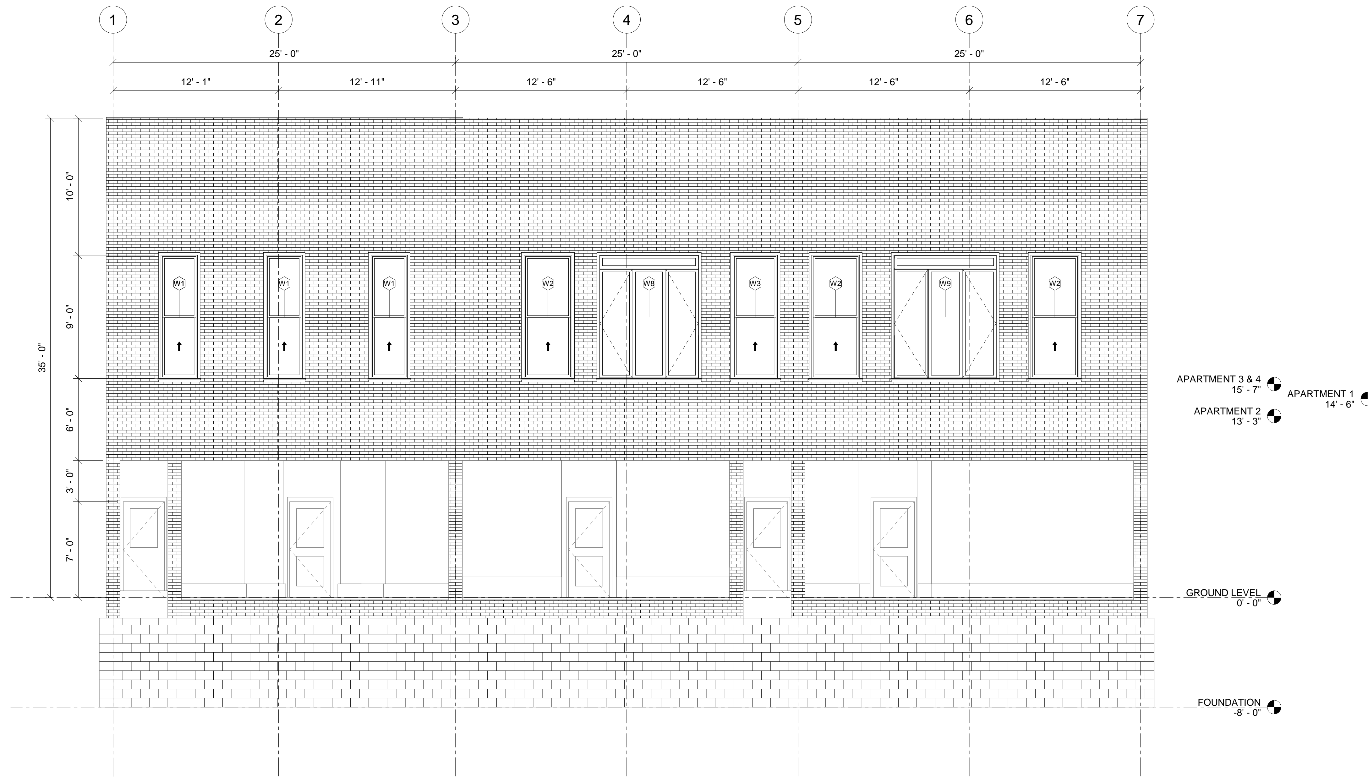
SE1 NORTH ELEVATION PLAN 1/4" = 1'-0"
